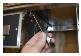
Slide the rail all the way to the end of the over-shelf so the Chilled Rail can be plugged in.
