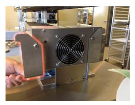
Lift the Chilled Rail into position underneath the overshelf. Tilt the rail so that the mounting bracket fits on the lip of the over-shelf.
