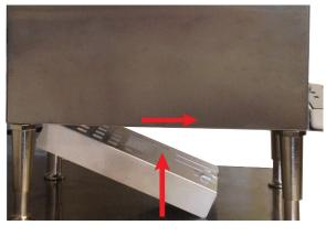
4. A "click" should be heard. Insert bin. If bin does not slide freely the creamer legs may need to be adjusted. Make sure bin guide is secure before leaving machine for use.
